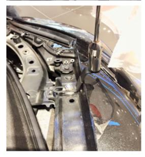
3. Measure the angle and length of the bevel required for the Z-Base.
