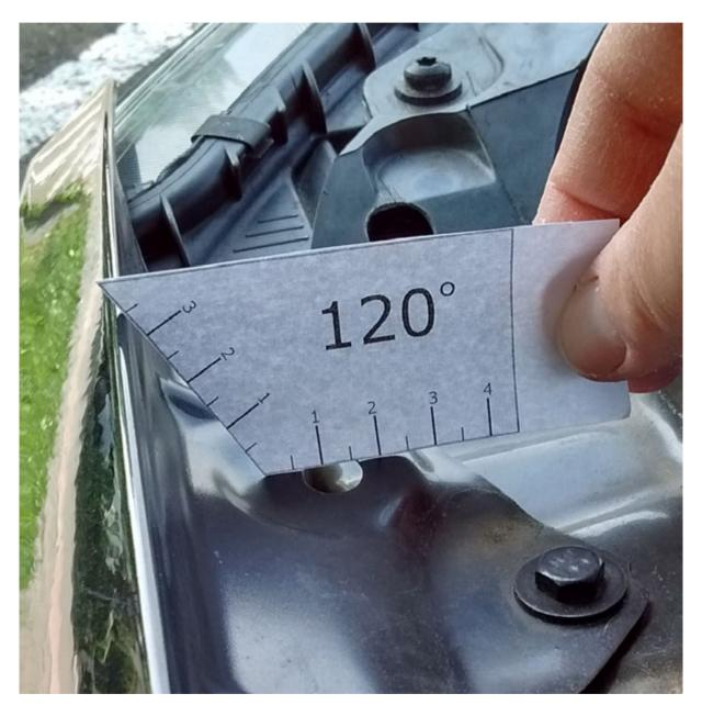
Example: An angle of  $120^{\circ}$  works best, with a bevel length of at least 4 cm, ideally 5 cm, to allow enough space for the screw.
